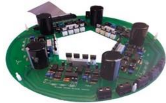
A proof-of-principle multi-level cascaded H-bridge inverter
